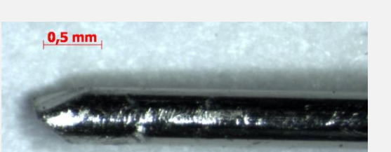
Fig. 2: Electrodes before and after a 2h inclined-plane-test with DC+
