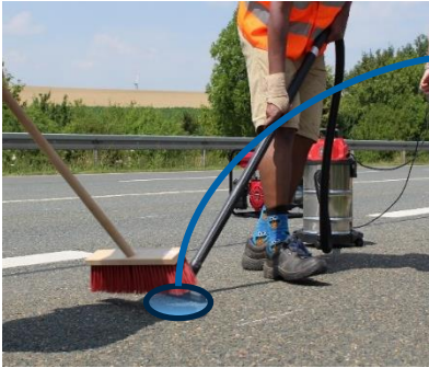
Fig. 3: Sampling with a vacuum system and a broom.
